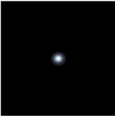
Figure 4.4: Top: Ray diagram of light emanating from a point source through an objective to the image plane. Because the objective collects only a portion of the spherical wave-front, light rays combine in a constructive and destructive fashion yielding the diffraction limited Airy pattern. Bottom left: Light emitting point source, expanded for clarity. Bottom right: Resulting image of the point source, now convolved with the point spread function of the imaging system.
