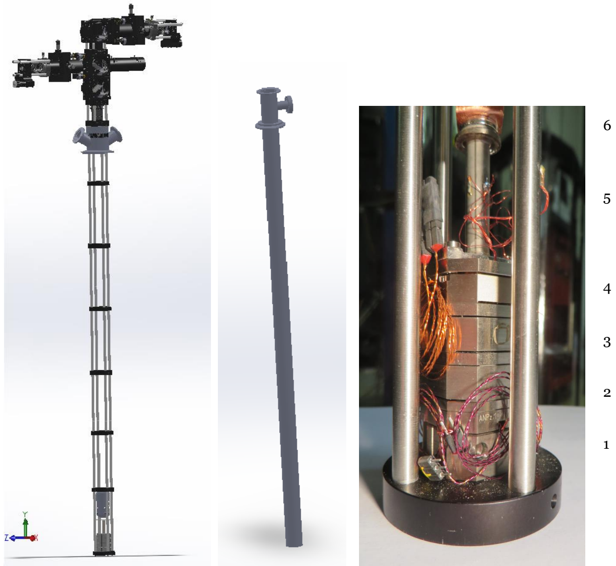
Figure 4.6: Left: The complete CTCSM, microscope head and the optical insert. Samples sit below the objective atop the positioners at the base of the optical insert portion of the CTCSM. Center: Insert tube that houses the optical insert when the microscope is used within the cryostat. Right: Close-up of the sample stage and piezo actuators used for coarse positioning and the raster process. Components as numbered 6. sample stage, 5. PI PT 130.14 piezo tube (raster scan), 4. ANSxy100lr (new raster scan positioner), 3. ANPx101 (X direction), 2. ANPx101 (Y direction), 1. ANPz101 (Z direction).
